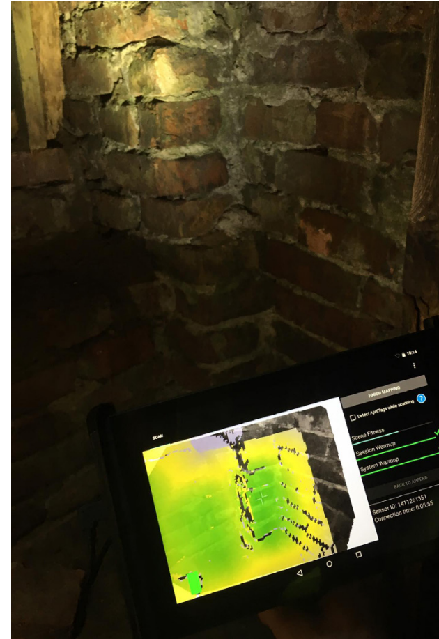
3D model of an architectural detail obtained via 3D optical scanner; produced and rendered by Przemysław Kluźniak. Photo credit: Natalia Romik.
