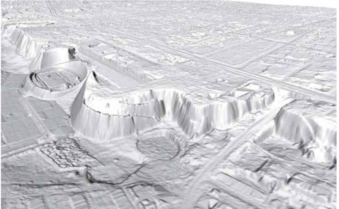
Numerical model of the escarpment area in the vicinity of the Warszawianka complex, Head Office of Geodesy and Cartography
