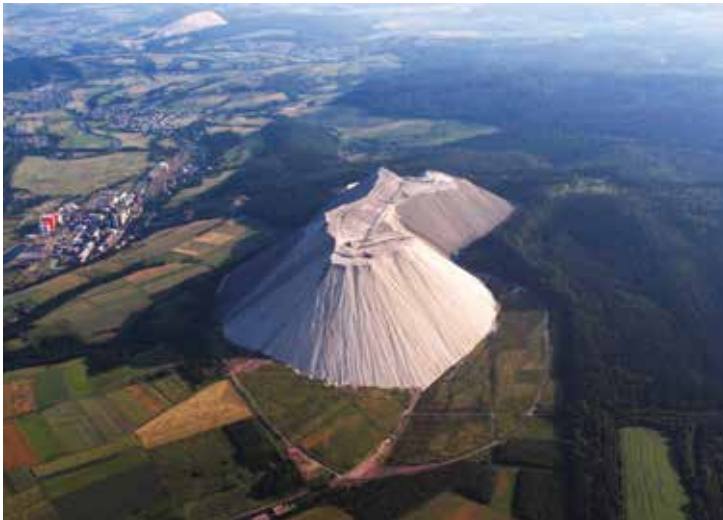
Monte Kali — a spoil heap of 188 million tonnes of salt, a waste product of local potash mining and processing, Heringen, Germany; photo: Wolkenkratzer, Wikimedia Commons, CC 0
